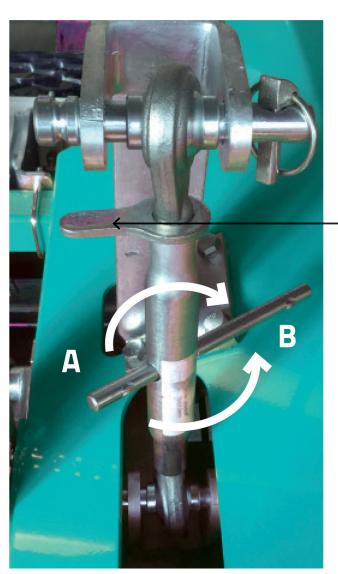
Caution! After adjustment please tighten the clamping screw again.
