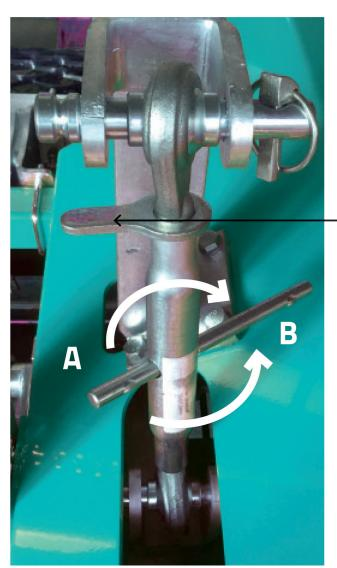
Caution! After adjustment please tighten the clamping screw again.
